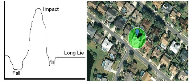
Fig. 1. The left image is an example of the total force applied to a tri-axis accelerometer during the course of a fall. The upper and lower thresholds can be adjusted based on the height, weight, and activity level of the user. The image to the right is a Google Map image depicting a variable radius in which a person with dementia should reside.
